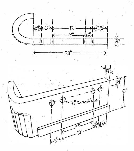
BLADE AND CURB GUARD DIMENSIONS: The following diagrams are to be used as a guide by the vendor. The vendor shall be responsible for verifying bolt spacings and dimensions with the plow manufacturer.
