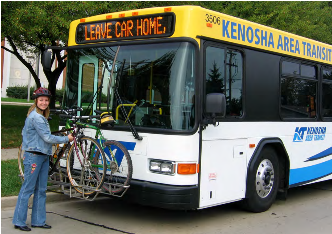
Figure 48. Most of Kenosha Area Transit's standing routes have buses equipped with bike racks.
